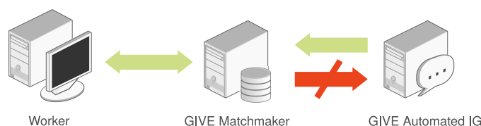
Figure 6.3: Network connectivity for our pipeline. The GIVE Matchmaker is on the public internet, while the GIVE Automated IG resides in a private network. Port forwarding is required to allow communication between them.
